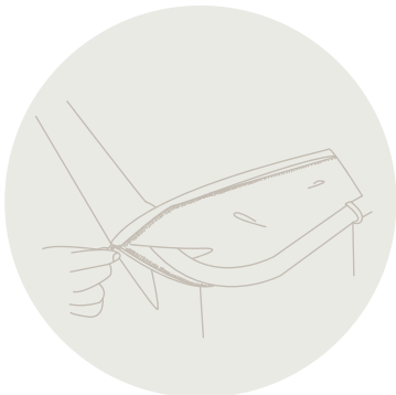
STEP 1 Unzip the lining at top and detach from Top Support Frame.
